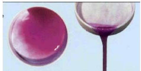
Score 3: Very definite gelling – no separate fluid. Difficult to shake mixture
